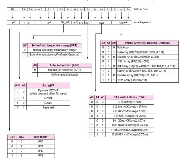
**Note1:** BA2, A5, A8, A11 ~ A15 are RFU and must be programmed to 0 during MRS. **Note1:** The Rtt\_WR value can be applied during writes even when Rtt\_Nom is disabled.
