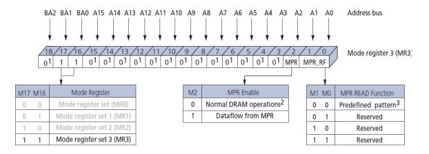
**Note1:** MR3[18 and 15:3] are reserved for future use and must all be programmed to 0. **Note2:** When MPR control is set for normal DRAM operation, MR3[1, 0] will be ignored. **Note3:** Intended to be used for READ synchronization.
