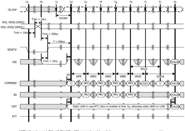
NOTE 1: From time point "Td" until "Tk" NOP or DES commands must be applied between MRS and ZQCL commands.
