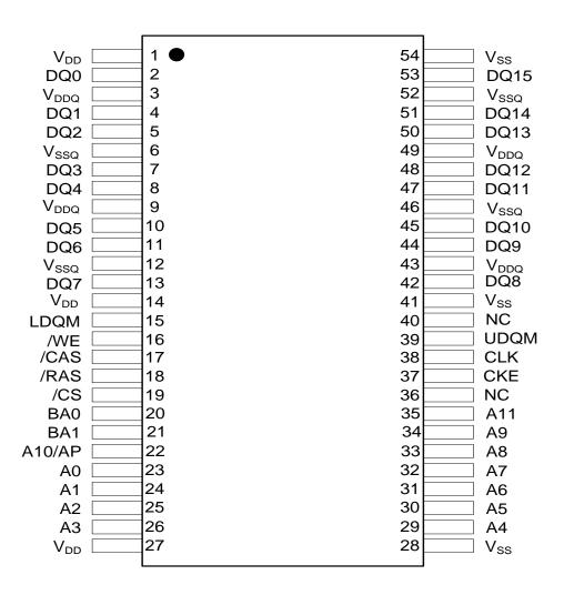
54pin TSOP-II / (400mil × 875mil) / (0.8mm Pin pitch)
