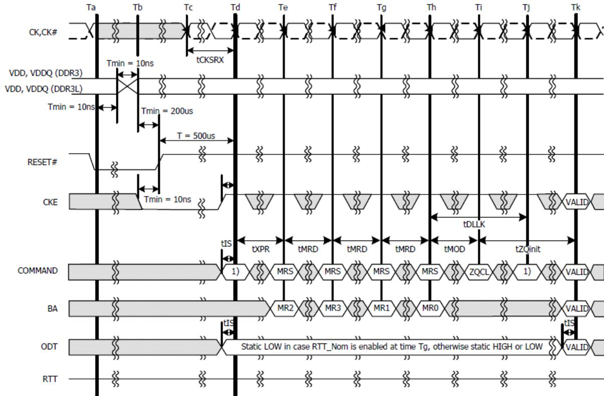
NOTE 1: From time point "Td" until "Tk" NOP or DES commands must be applied between MRS and ZQCL commands.
